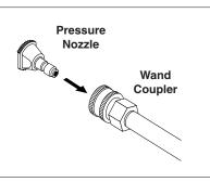
**STEP 6:** Pull the spring-loaded collar of the wand coupler back to insert your choice of pressure nozzle.
