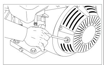
STEP 9: Pull the starter grip. If the engine fails to start after 2 pulls, squeeze the trigger gun to release pressure and repeat step. Return starter gently. After the engine warms up enough to run smoothly, move choke to run position and throttle to fast position. CAUTION: Small engines may kick back. Do not hold pull starter grip tightly in hand
