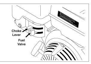
**STEP 6:** Move the choke lever to the "Choke" position (on a warm engine, leave the choke lever in the run position). Move the choke lever to the "Closed" position. To restart a warm engine, leave the choke lever in the "Open" position.
