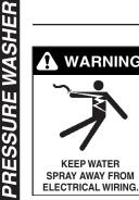
WARNING: Keep wand, hose, WARNING and water spray away from electric wiring or fatal electric shock may result.
