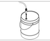
STEP 1: Remove detergent suction tube from container and insert into one gallon of fresh water. Slide nozzle forward for low pressure or to connect black detergent nozzle. Pull trigger on spray gun and siphon water for one minute.
