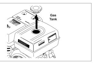
**STEP 3:** Fill gas tank with unleaded gasoline. Do not use leaded gasoline.
