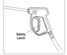
WARNING! Never replace nozzles without engaging the safety latch on the spray gun trigger.
