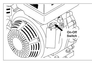
STEP 8: Turn the engine switch to "On" position. On Briggs engines, move the throttle lever to "Fast" position, shown on the engine as a rabbit.
