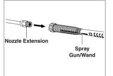
**STEP 5:** Attach nozzle extension to spray gun/wand. Tighten both by hand.
