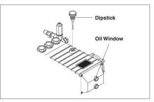
**STEP 1:** Check engine oil level. Oil level should be level with the bottom of the oil filler neck. Be sure the machine is level when checking the oil level. (Refer to the engine's operating manual included with machine.) We recommend that the oil be changed after the first 5 hours of use, then once every 50 hours. **Note:** Improper oil levels will cause low oil sensor to shut off engine. **IMPORTANT! Do not run engine with high or low oil levels as this will cause engine damage.**
